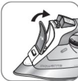
**IMPORTANT** Before filling the water tank, unplug the iron and set the steam control to dry position
