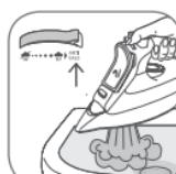
Fill the water tank with untreated tap water up to the max mark and heat the iron to the temperature. Unplug the iron and hold it over a sink horizontally. Hold the steam control into the Anti Calc position : steam will now begin to build up. After a few seconds water will emerge from the soleplate, rinsing dirt and scale particles out of the steam chamber.
