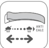
Unplug the iron, pour away remaining water and set steam control to . Open and close the steam control several times to prevent the valve hole into the steam chamber from scaling or blocking up.
