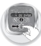
3- When you have finished entering all your settings, press the "start" button (B7). When your appliance is using cooking mode, the red indicator light (B3) lights up to inform you that cooking has started. When the program has started, you have the possibility of stopping the appliance at any time by pressing the "stop" button.
