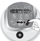
2- Then adjust the setting(s) using the +/- selector (B6). For safety reasons, it is not possible to set a temperature without setting a cooking time.
