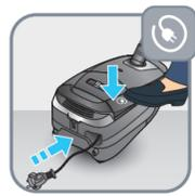
**EN** To switch off the vacuum cleaner, press the ON/OFF button after use. Unplug the vacuum by pulling it out of the socket. To rewind the cord, unplug the cord and press the rewind button until the cord is totally stored.
