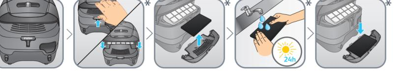
**EN** Open the back rear flap by lifting it up. The black foam filter is washable. Only use clear water to wash it. Let it dry 24 Hours before putting it back.
