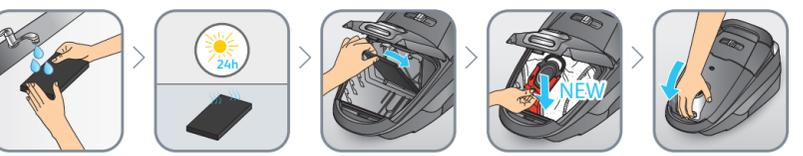
**EN** Wash it with clear water and let it dry for 24 hours. Put it back in its original place. Put a new hygiene+ bag. Close the front rear flap.
