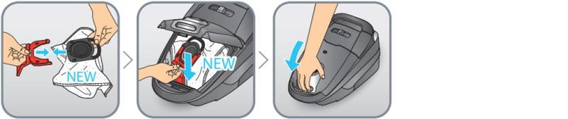
**EN** Get a new Hygiene+ bag and clip it on the bag holder by following the arrows. Then put it back on its original place. Close the rear flap.
