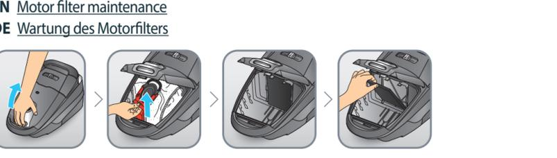
**EN** Open the front rear flap by lifting it up while pressing the strip. Remove the Hygiene+ bag. Remove the motor filter.
