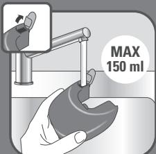
**EL** Fill the water tank with a maximum of 150 ml of untreated tap water.
