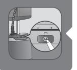
**EN** Long push the ON/OFF button in order to switch off the appliance.
