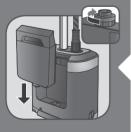
Screw back the cap and place the water tank back in the appliance.
