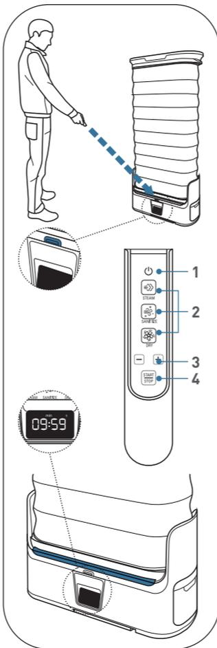
Point the remote control at the infrared receiver..
