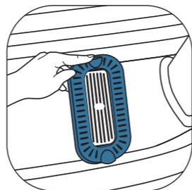
SLift out the shelf, remove the filter and remove any residue that may be there with a sponge.
