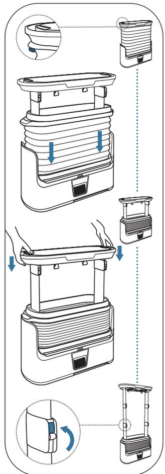
Pull the switch for locking/unlocking the shutter to lower it.
