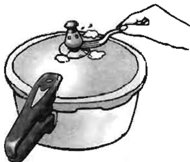
Figure 13. Check for Pressure
