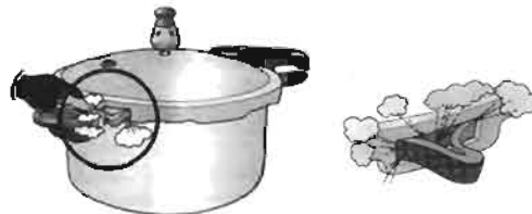
Figure 8. Overpressure Safety Window
