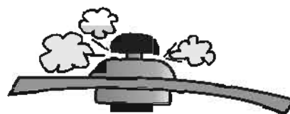
Figure 6. Overpressure Valve Releasing Steam
