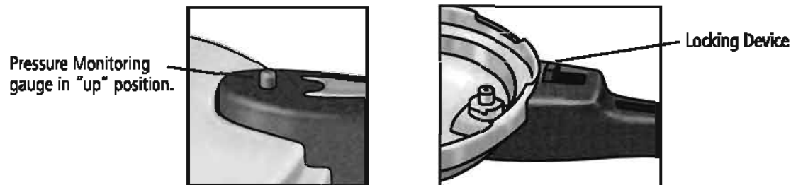
Figure 9. Pressure Monitoring Gauge and Locking Device
