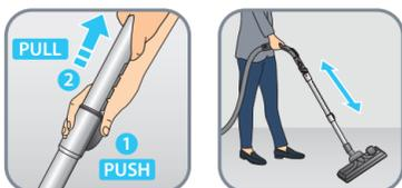
**EN** To adjust the telescopic tube at your height : push the telescopic button and pull the two parts of the tube in opposite direction.
