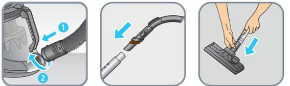
**EN** Insert the hose inside the connector and turn it clockwise until it is locked. Insert the handle into the tube. Insert the tube into the floorhead.
