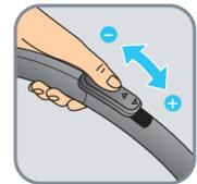
**EN** To open the air inlet and reduce the suction power, push the slide button up. To close it and increase the suction power, push it down.
