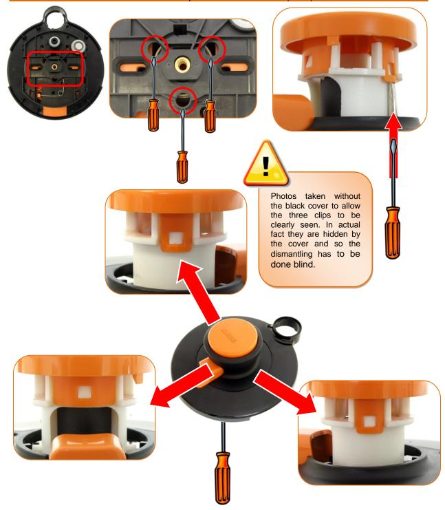
When dismantling the module cover blind, if one or more of tabs breaks during dismantling, you will need to change the cover.
