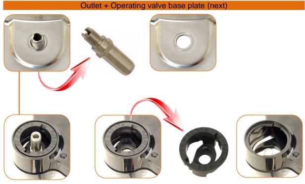
To refit it, apply a torque of 10.35N.m ±3,5 or 1.02m.Kg
