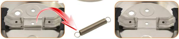
To refit the return spring for the jaws, it is essential to place it on the hooks located opposite the safety and operating valve holes, as shown in the photo beneath.
