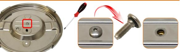
If the central screw seal is damaged, simply replace the screw. For refitting, apply a torque on the screw of  $4N.m \pm 1$  or 0.41m.Kg
