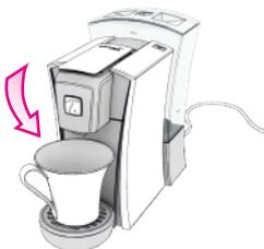
Press **7** until water tank is empty and discard the descaling agent.
