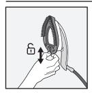
Before you remove or attach the brush, switch off the appliance and allow it to cool down for 1 hour.
