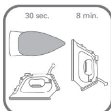
If your iron is equipped with auto-off and the iron is not moved while it is plugged in, an internal safety switch will turn it off.
