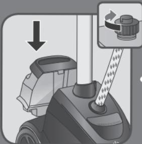
**EN** Fully tighten the water tank cap and insert tank back in appliance.
