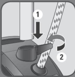
**EN** Insert the pole in the housing & then lock.
